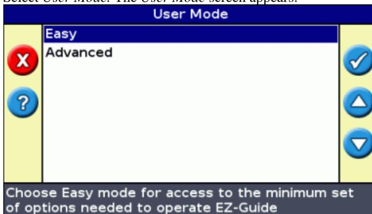
3. Select Advanced or Easy and then press
