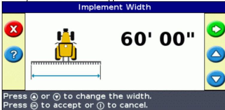
1. Press or to adjust the implement width and then press . The *Overlap/Skip* screen appears.
