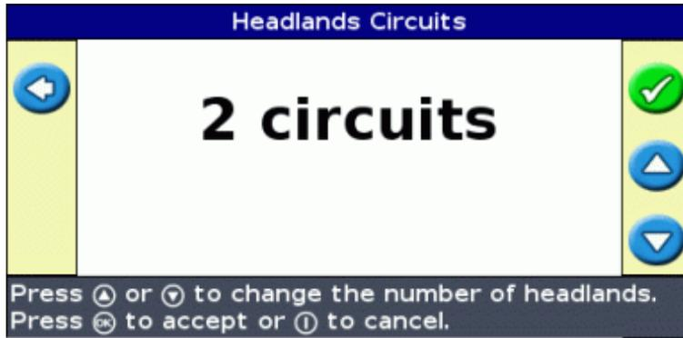
1. On the *Headlands Circuits* screen, press ▲ or ▼ until the screen displays the required number of circuits.
