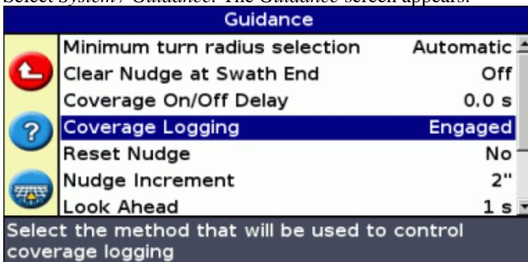
5. Select *Coverage Logging* and then press
