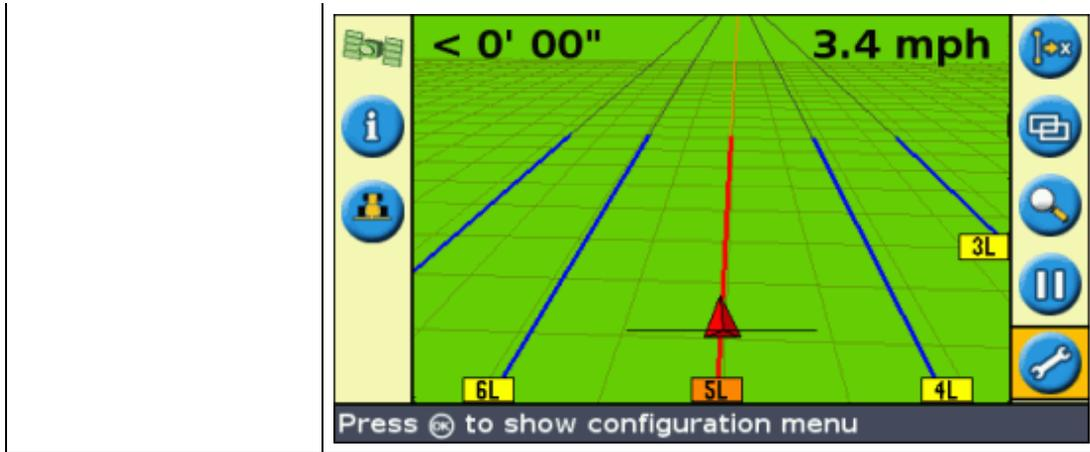
*Note: When the vehicle is on a guidance line, the line extends 1 km (0.6 miles) before Point A and 1 km beyond Point B. This makes it easier to see where the next swath is, and to get online after the turn.*
