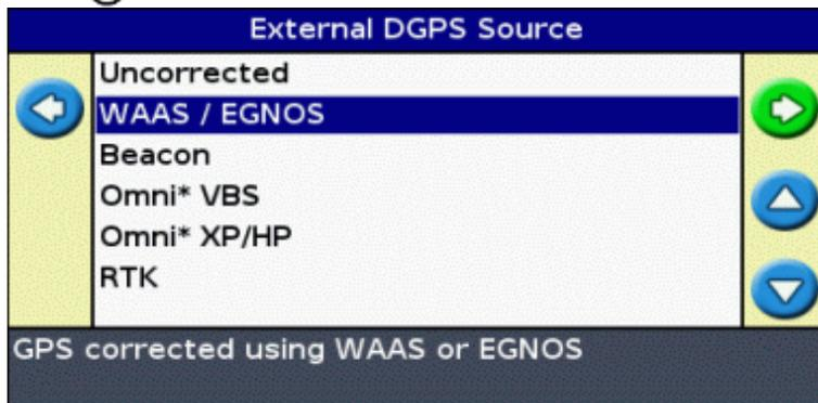
6. Select the appropriate correction source and then press **OK**. The wizard for that correction type appears.
