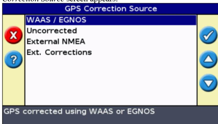
2. Select the appropriate correction method and then press **OK** . The *GPS Source* screen reappears. The correction appears as the Source.
