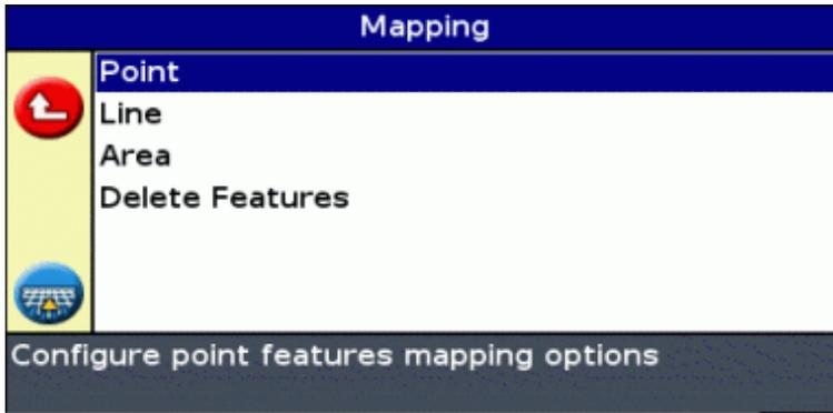
3. Press to select Point, Line or Area and press to display the configuration screen for the feature type.
