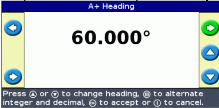
The default heading is the same as the previous AB Line. This pattern is useful for when you need guidance exactly parallel to the last AB Line, for example when:
