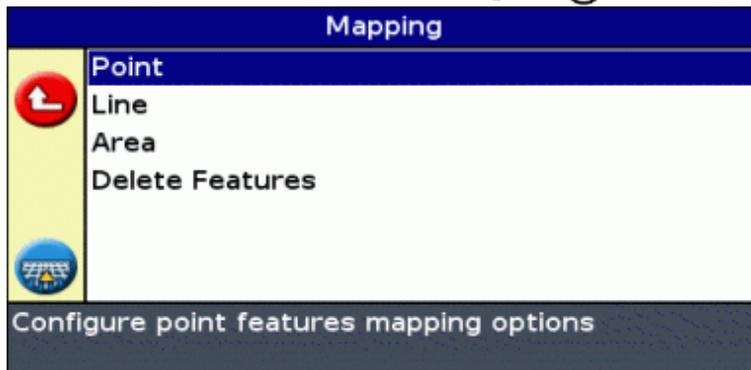
3. Press **▼** to select *Point*, *Line* or *Area* and press **OK** to display the Point, Line or Area feature configuration screen.
