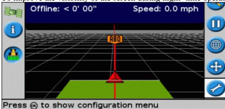
To change to night mode, select *Configuration / System / Display / Color Scheme* and select *Night Mode* .
