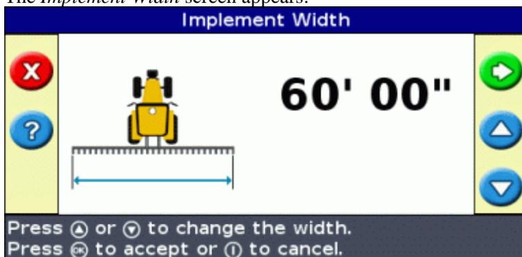
1. Press **[Up/Down]** to adjust the implement width and then press **[OK]** . The *Overlap/Skip* screen appears.
